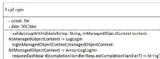
Gambar 10. Class Diagram LogLogin
