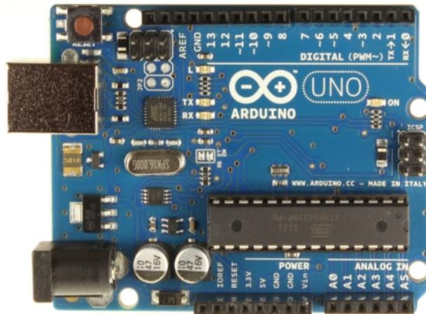
Gambar 1. Microcontroller Arduino Uno
